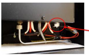
NB: A TCO usually only trips if there is a problem. If it trips again the Smoke Screen should be checked for faults before further use.
