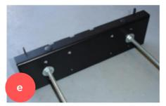
Prepare the Smoke Screen by fitting the angle brackets. Fix the required length of M8 threaded bar to the bracket using 4 x nuts and 4 x 25mm washers.
