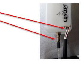
Connect the monitoring cable and feed pipe to a new fluid reservoir. Insert the reservoir into the fluid compartment top first. Make sure the label on the reservoir is on the outside of the Smoke Screen. This orientation ensures that the fluid feed is correct for both upright and face-down installations.
