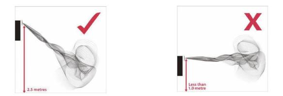
The optimum wall mounting position for the Smoke Screen is 2.5 metres above the floor facing the area to be protected and using the 30-degree angle nozzle. The maximum recommended mounting-height above floor level is 3 metres, the minimum is 1 metre and there should be no obstacle within 1 metre of the smoke output nozzle. Also, leave a minimum of 150mm clearance to the ceiling.
