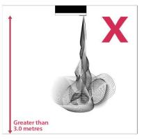
The optimum ceiling mounting position for the Smoke Screen is 2.5 metres above the floor facing the area to be protected and using the standard straight nozzle. The maximum recommended mounting-height above floor level is 3 metres, the minimum is 1 metre and there should be no obstacle within 1 metre of the smoke output nozzle.
